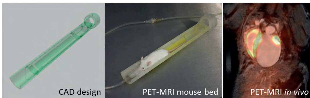
Figure 4: The PIX PET-MRI bed: From design to application After defining the specific requirements for a PET & MRI compatible mouse holder 3D models of the common bed (left) were designed and finally manufactured (K. Schäfers & L. Frohwein). The shown PET-MRI mouse bed (middle) provides integrated heating pipes, channels for anaesthesia and a connector for existing bed holders. First PET-MRI image of a myocardial infarction in a mouse in vivo using the novel PET-MRI bed (right). PET reveals FDG uptake in viable myocardium (yellow color) delineating a huge myocardial infarction in the left ventricle which correlates with thinning of the left ventricle as shown by MRI.
