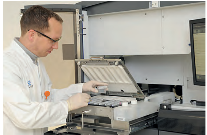
Next Generation Sequencing on a Life Technologies SOLiD 5500xl sequencer
