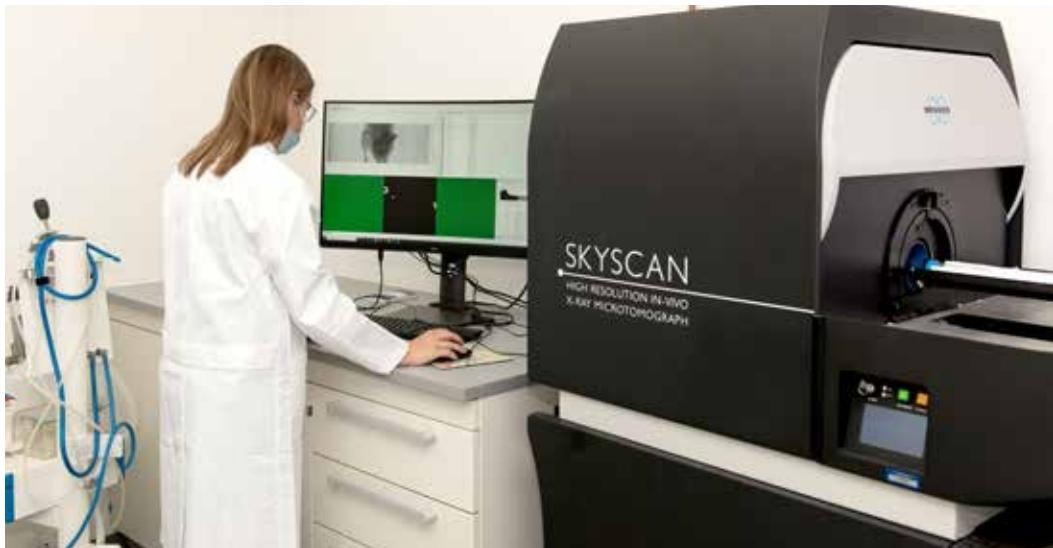
MicroCT X-ray micro computed tomography imaging used to evaluate bone microstructure during murine osteoarthritis, joint injury and inflammatory arthritis models via 3D image reconstruction and quantitative analysis
