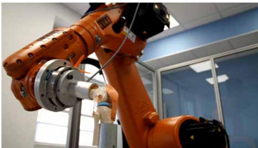
Industrial robot for experimental analysis of joint kinematics, demonstrated by the example of an artificial knee
