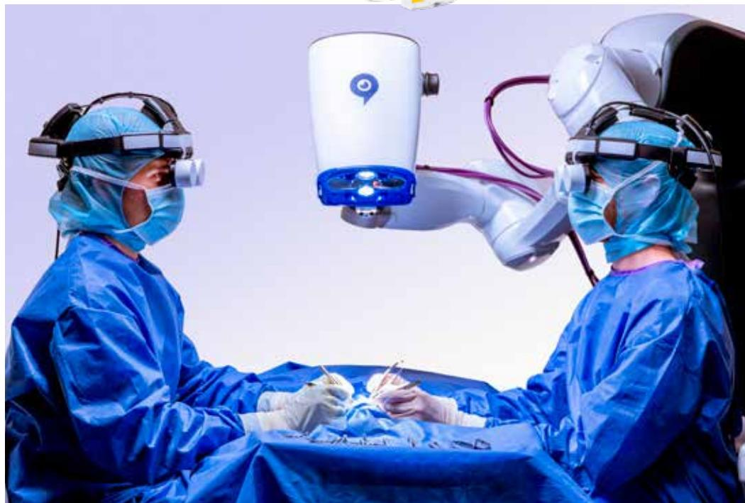
*Top row: Symani robotic microsurgery system with remote surgical instrument control (Photos: MMI S.P.A), Bottom row: BHS robotic microscope with augmented reality headsets (Photo: BSH Technologies GmbH)*
