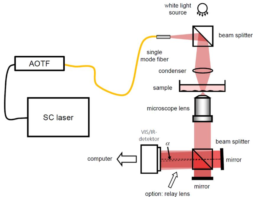
**Figure 1.** Concept for multi-spectral digital holographic microscopy.  $\alpha$ : off-axis angle between object and reference wave, AOTF: Fiber coupled acousto-optic tunable filter, SC laser: fiber-coupled super continuum laser source (adapted from [27]).
