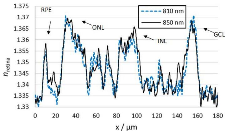
**Figure 4.** Representative calculated integral refractive index  $n_{\text{retina}}$  of the retina along the cross-section indicated with dashed lines in Fig. 3a for the two wavelengths  $\lambda = 810$  nm and  $\lambda = 850$  nm (adapted from [37]).
