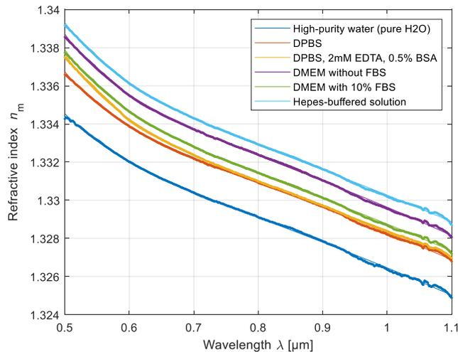
**Figure 2.** Refractive index dispersion retrieved in the spectral range from 500 nm to 1100 nm from measurements on different physiological buffer solutions at a temperature of 22°C. (adapted from [33]).
